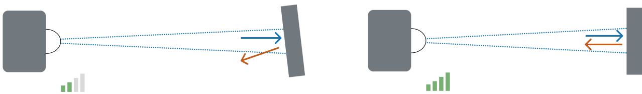
Align sensor perpendicular to target for better signal strength
